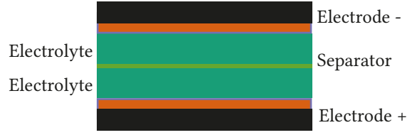
Fig. 3.12 Structure of a supercapacitor.
